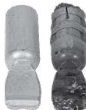
Uncrimped Good Contact
